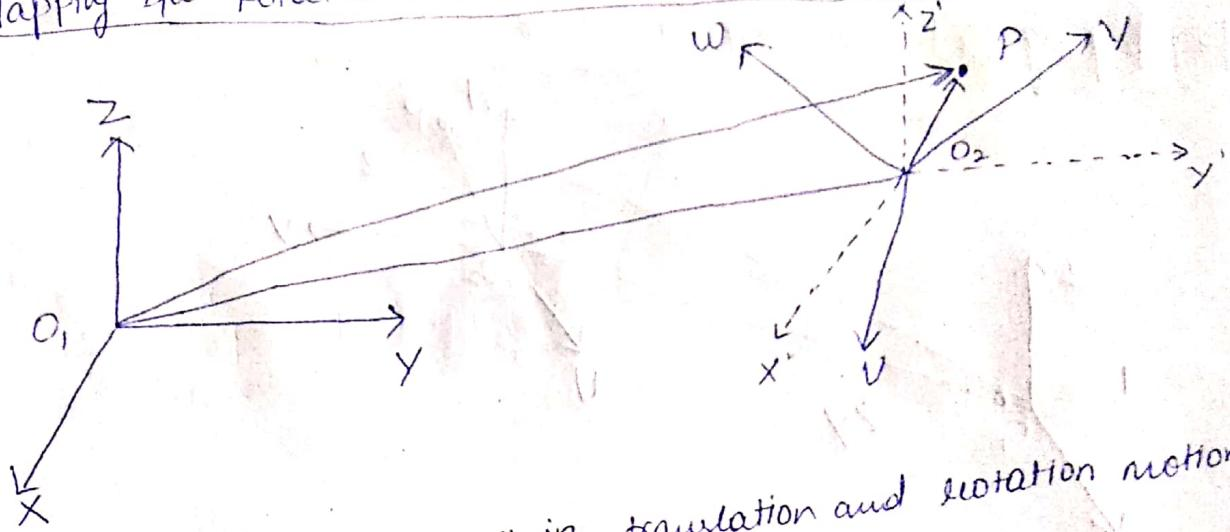
In this frame 2 moves in translation and rotation motion with respect to 1.
