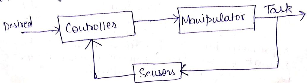
The positions, velocity, forces and torques are measured by sensors and based on these measurements and the desired behaviour, the controller determines the input so that the end effector carries out the desired task as closely as possible.
