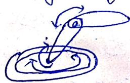
(v) SCARA robot  $\div$  SCARA Robot has 3 rotary motion & 1 linear motion. It is mainly use for pick & place of any object.
