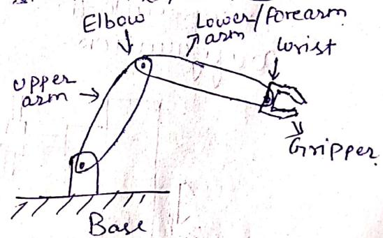
→ Robotic arms are used in industries where humans are not able to work i.e., high temperature, polluted air zone, heavy weight lifting etc. Robotic arm also used for perform a task accurately in various environment.
