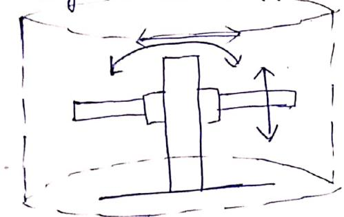
It consist of 2 Ls Prismatic joint & a revolute joint. The arm end is thus capable to sweep cylindrical space. The work space of cylindrical configuration is hollow cylinder.
