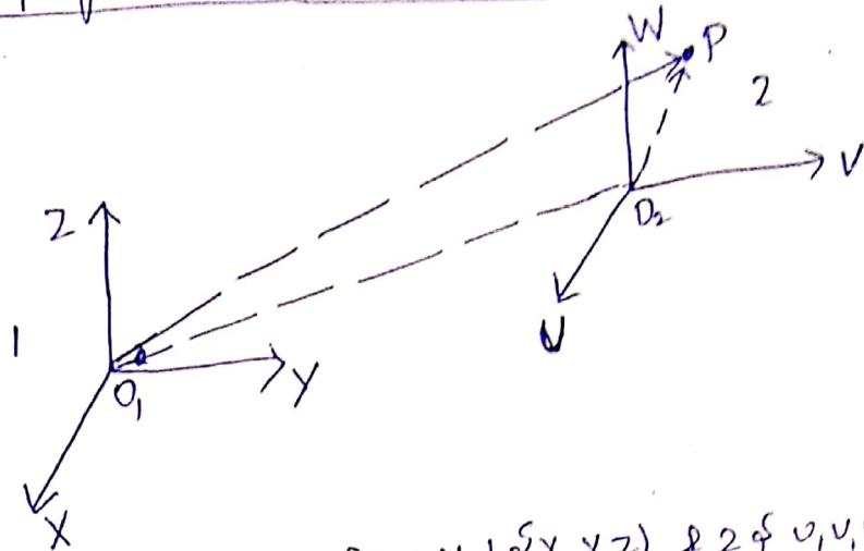
Consider there are two frames  $1\{x, y, z\}$  &  $2\{v, v, w\}$  having origin point  $O_1$  &  $O_2$  respectively. In this frame, 2 moves in translation motion with respect to 1.
