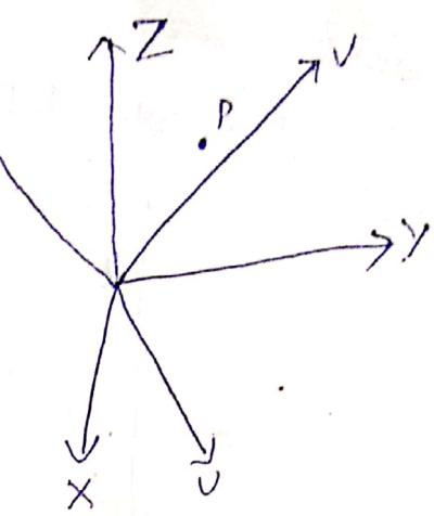
Similarly, when we find the description of point P in Frame 2 when description of Point P in Frame 1 is known. Then,  ${}^2P = {}^2R_1 {}^1P$
