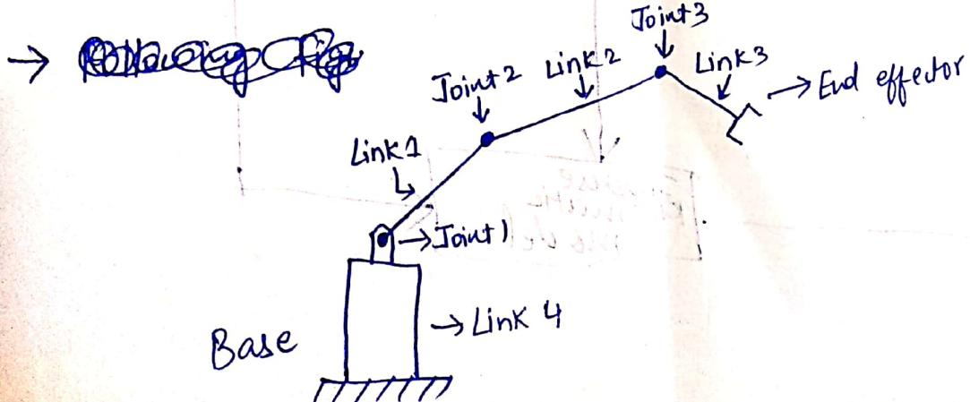
→ Above figure is of 3-DOF Manipulator arm in an open kinematic chain having 3 revolute joint & 4 links. So, n-DOF manipulator arm consists of  $(n+1)$  link &  $n$  joints.
