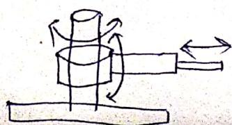
(iv) Joined Arm Robot: This type of robot only performs rotary motion. This type of robot have 3 rotary motion.
