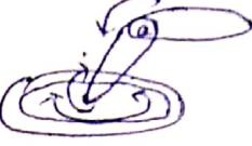
(v) SCARA Robot: SCARA Robot has 3 rotary motion & 1 linear motion. It is mainly used for pick & place of any object.
