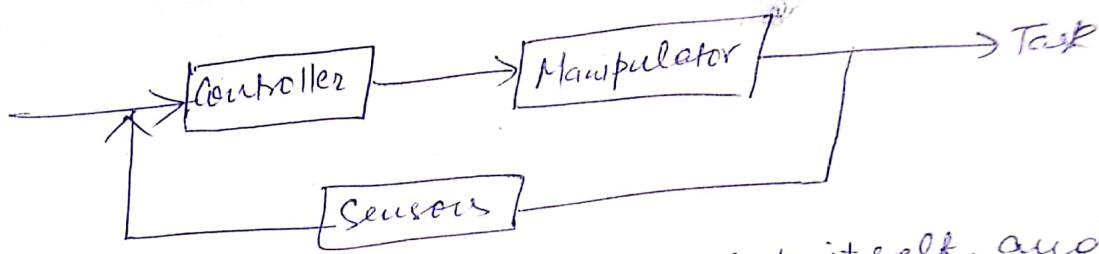
External sensors are external to the robot itself, and are used when we wish to control the operation of robot.
