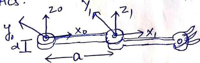
$\theta$  = A rotational angle between two links, about the  $z$ -axis
