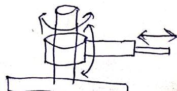
(iv) Jointed Arm  $\div$  This <sup>robot</sup> type of robot only performs rotary motion. This type of robot have 3 rotary motion.
