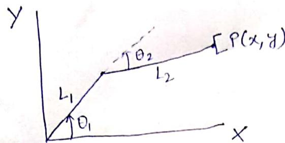
There are two links  $L_1, L_2$  and assume that the joint angles are  $\theta_1, \theta_2$  and the coordinates of end effector point  $P(x, y)$  is given. From simple geometry analysis of this manipulator, it is possible to compute coordinates  $(x, y)$  from the joint angle  $\theta_1$  &  $\theta_2$ .
